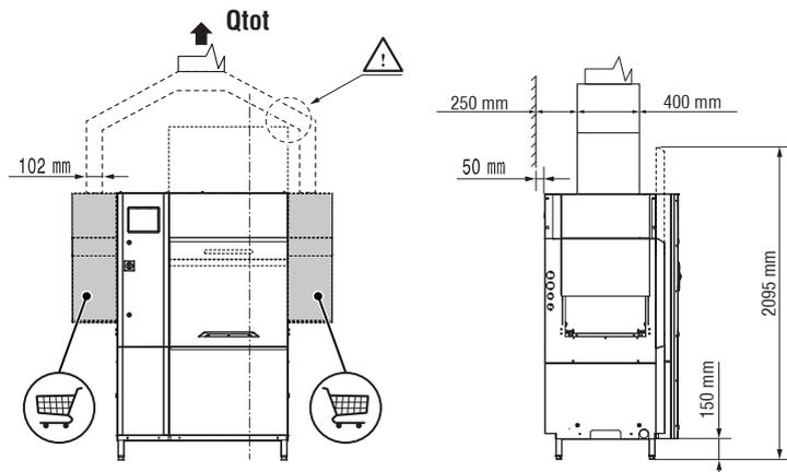
All exhaust hoods must be dimensioned and installed according to local regulations and industry standards which may differ from the recommendations herein suggested. Electrolux Professional is not liable for any failure in complying with local design standards.
